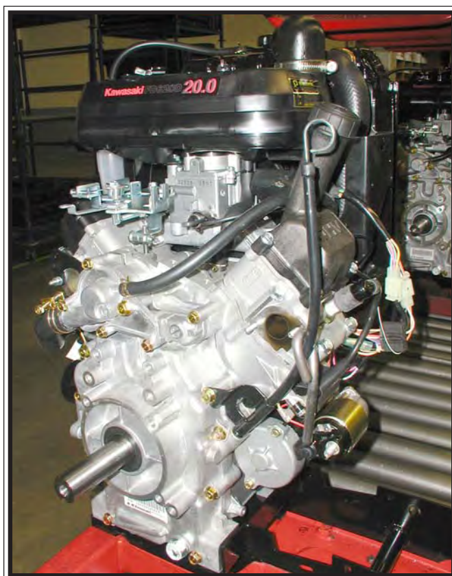
Kawasaki FD620D Liquid Cooled 20 H.P OHV
